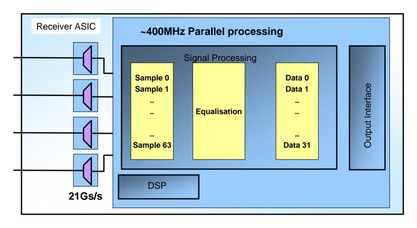
• Once the signal is digitized, CMOS technology can process the data efficiently in parallel.
