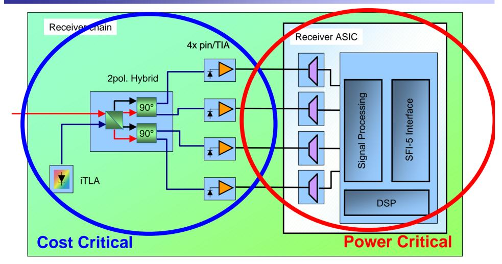
Building blocks are common to 40/100G CP-QPSK / n-QAM / OFDM
