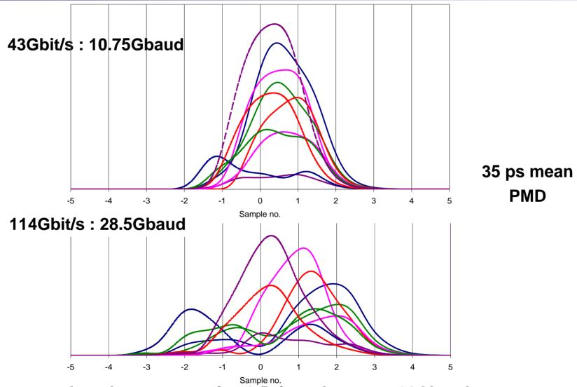
Impulse response is ~2.5 times longer at 28Gbaud Rate of Polarisation change is the same
