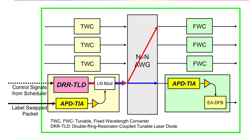
N×N non-blocking switch for packet-level switching
