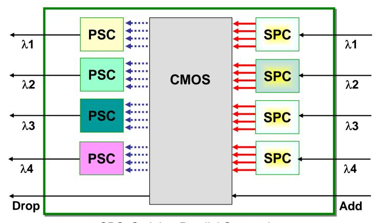
SPC: Serial-to-Parallel Conversion PSC: Parallel-to-Serial Conversion
